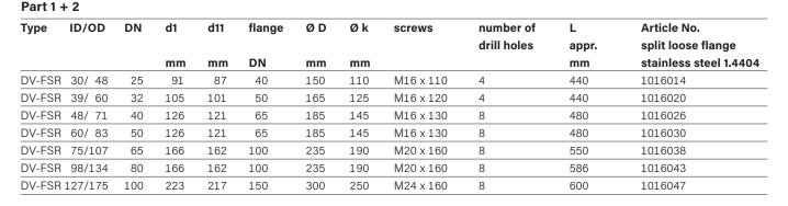
Screws and nuts are not included in the delivery volume. Only BRUGG solder Type BRL 8.50.34 may be used!
