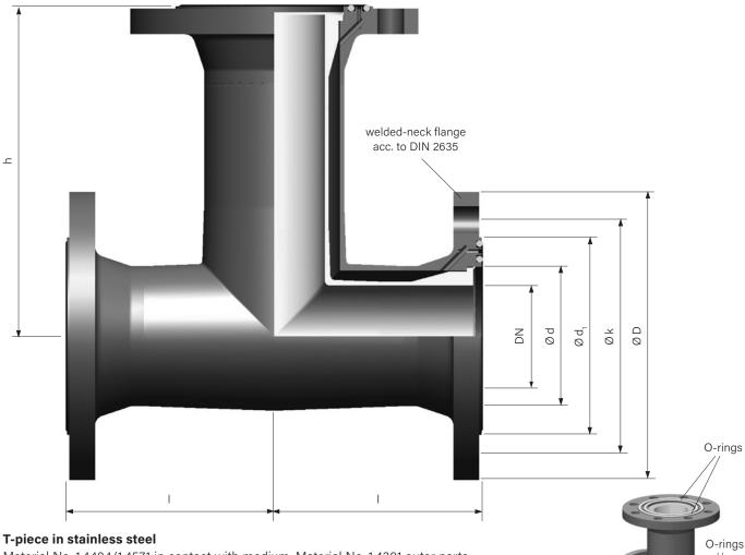
Material No. 1.4404/1.4571 in contact with medium, Material No. 1.4301 outer parts The monitorable T-piece with flanged connection is flanged together with monitorable connecting fittings with loose flange Part 1 (Worksheet FSR 4.216) or welded-neck flange.
