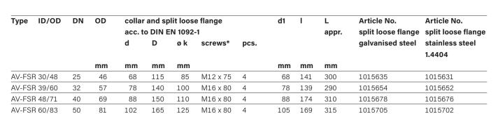
Screw length is given for the connector to a welding-neck flange acc. to DIN EN 1092-1. Screws and nuts are not included in the delivery volume.
