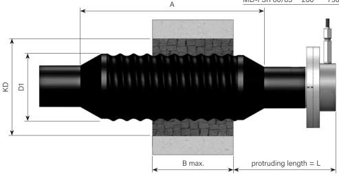
\* If walls are thicker, two wall ducts can be pushed inside one another.
