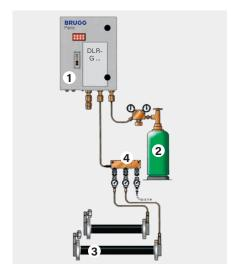
Positive pressure leak detector
