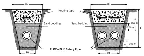
The routing tape is delivered by BRUGG and must be laid on site.
