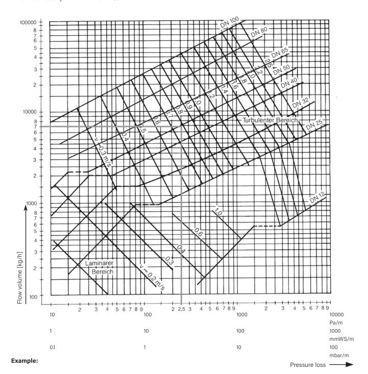
Pipe DN 50 With a flow volume of 7000 kg/h at a speed of c. 0.8 m/s the pressure loss is 2.5 mbar/m
