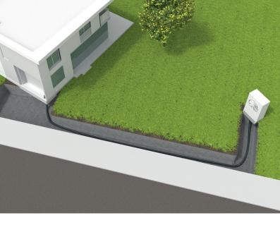
The innovative FLEXSTAR low-temperature system from BRUGG Pipes is a pre-insulated pipe system with maximum flexibility and stability for heat pumps or local heating networks.
