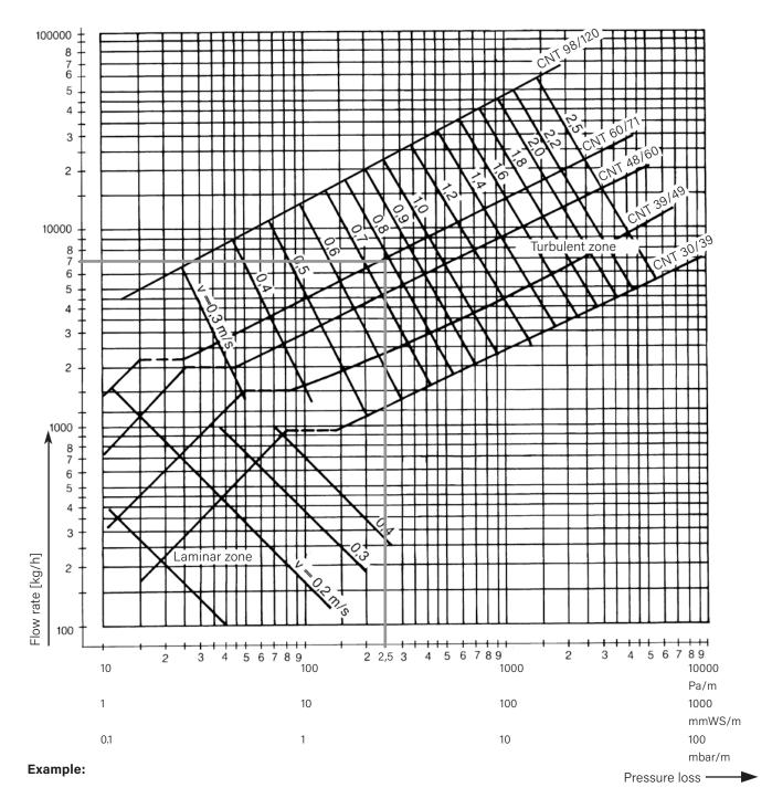
Pipe DN 50 Mass flow 7000 kg/h at a speed of c. 0.8 m/s pressure loss is 2.5 mbar/m
