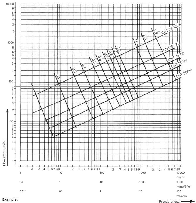
Pipe DN 50 Flow rate 80 l/min at a speed of c. 0.4 m/s pressure loss is 0.6 mbar/m
