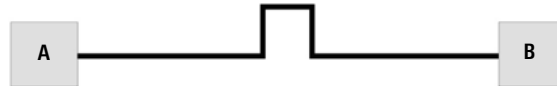
Figure 4 Straight pipe routing between two buildings, with expansion accommodated by U-bends within the pipeline.
