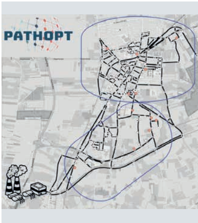
Figure 2. The Eeklo case, with the producer at the bottom of the figure. Consumers are the white (medium heat demand) and orange (high heat demand) dots, while the black lines represent the streets. Encircled are the two investment zones, the zone closest to the producer will be connected first
